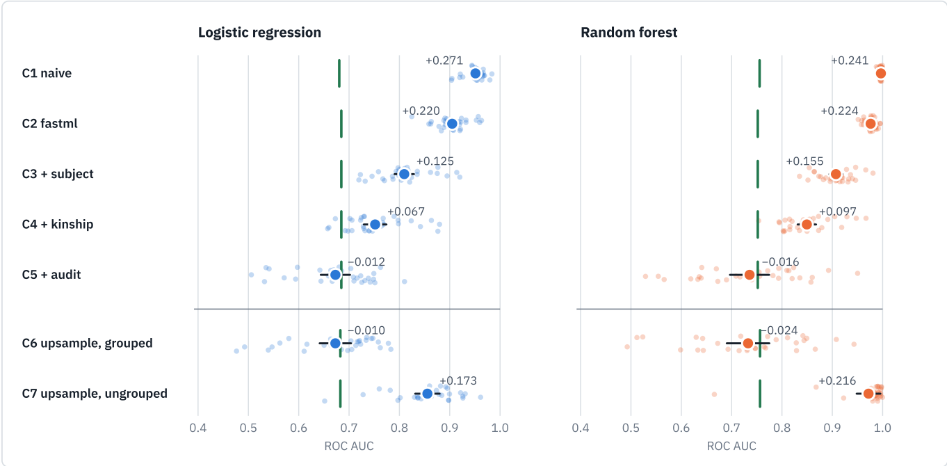
Figure 3. Cross-validated AUC under each configuration: faint dots show the 30 replicates, the large dot the mean, and the whisker the 95% t-interval of the mean. The short green tick marks the configuration’s mean external AUC (final model), and the label gives the mean paired bias. C1–C5 move the estimate toward the external value; among C1–C5 only C5’s interval covers it for both learners, and C6’s does as well. C6 shows that upsampling before honest folds is harmless when copies stay with their source; C7 shows that it is not when they scatter. Hover over a dot for its values.
